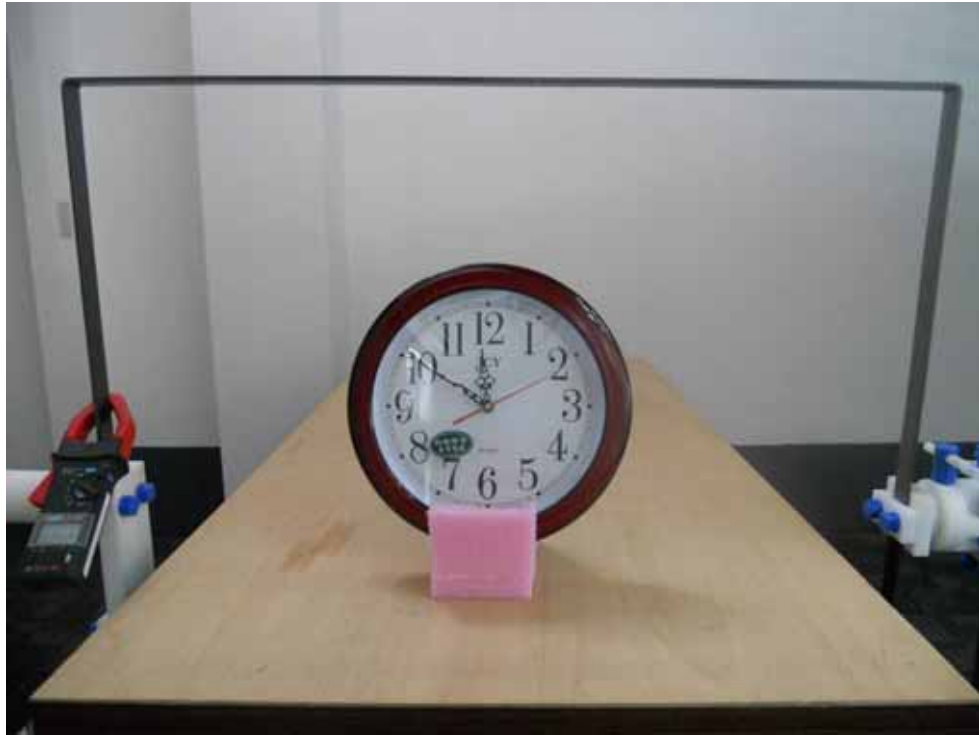
Picture 17:Power Frequency Magnetic Field Immunity.(12888S)
