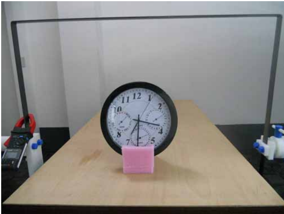
Picture 19:Power Frequency Magnetic Field Immunity.(12888SMP)
