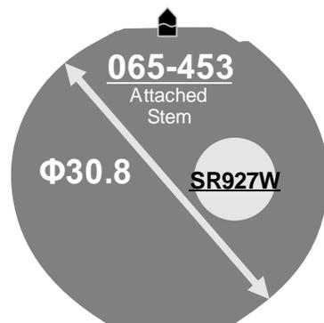
Battery consumption could be minimum by pulling out the stem
