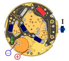
Setting stem in position I, calendar not in gear, 60 s measuring interval for rate and consumption:
