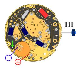
Setting stem in position III, 60 s measuring interval:
