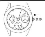
2.Push the crown back into the normal position in signal.
