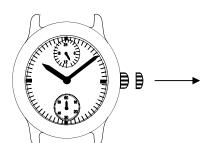
2.Turn the crown to set the hour and minute hands to the time. (Check that AM / PM is set correctly)
