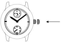
3. Push the crown back in to the normal position in accordance with a time signal.
