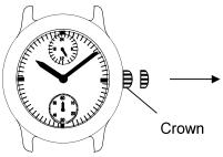
1.pull out the crown to the second click when the small second hand is at the 12 O'clock position.
